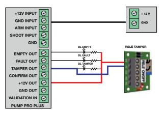
In case of an empty bag, the EMP LED (EMPTY) will switch on.
