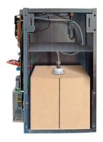
Insert the plastic bag in the compartment as shown in the picture
