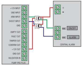
Compared to B diagram, this alarm central has only open collector outputs.
