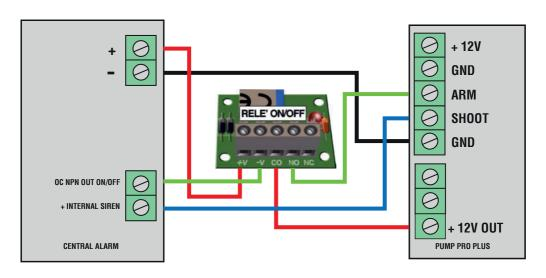
In the diagram above the control panel, as example, provides to UR Fog power supply between 11 and 14V DC 250 mA max. The ON/OFF output of this alarm is an Open Collector NPN opened when the system is off and it is stably closed to negative as long as the system turned on.
