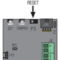
In order to make the reset the jumper P3 must be on the right position as you can see in the picture.
